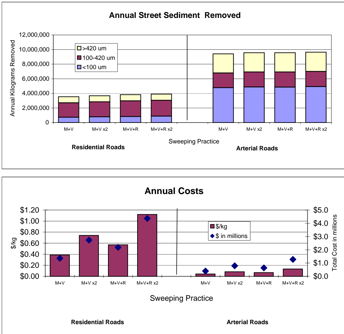
Figure 5 Comparison of Different Street Sweeping Practices - Annual Removal with One Spring Sweep
